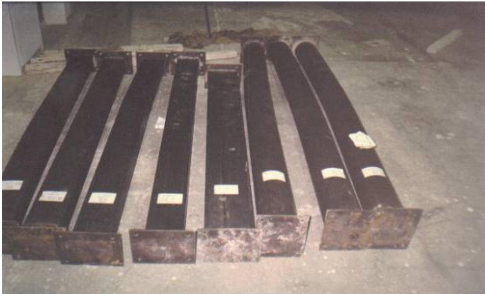
Figure 2 : Mode of Failure for Some of the Tested Columns
